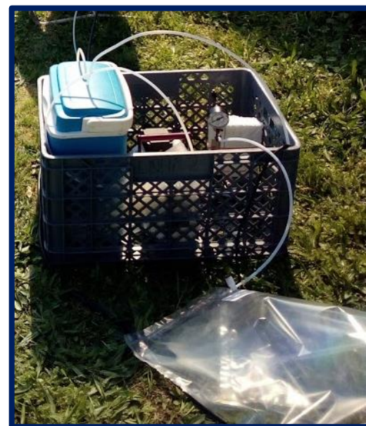
Tedlar bags to collect gaseous samples
