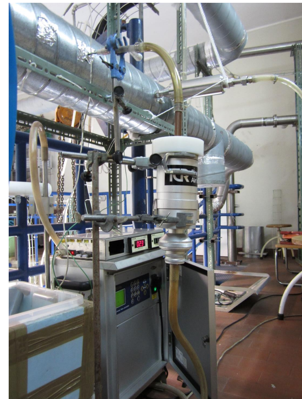
PM sampling in the dilution tunnel connected to the exhaust chimney
